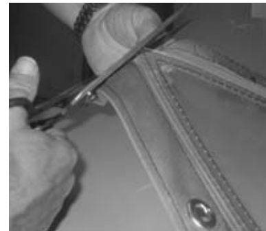
Cut the Ocean Clear at a 45° angle on the corners to eliminate sharp points.
